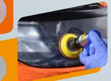
WET SAND WITH **NORTON SUPERFLEXIBLE Q775 DISC P3000** + SOFT INTERFACE
