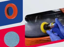
**DRY SAND WITH NORTON PRO PLUS SMART REPAIR A975 DISC P500**
