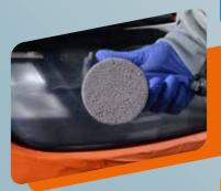
WET SAND WITH **NORTON SUPERFLEXIBLE Q775** DISC P1500 + SOFT INTERFACE
